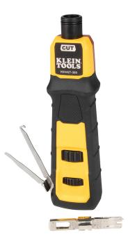
Premium performance, impact punchdown tool provides precise, reliable connections every time. Use to punch data cables into 66/110 panels and blocks. Terminate and cut wire in one step with the MIM (metal injection molding) precision ground combination 66/110 blade. The tool features the traditional punchdown-style form with a cushioned, non-slip handle.
