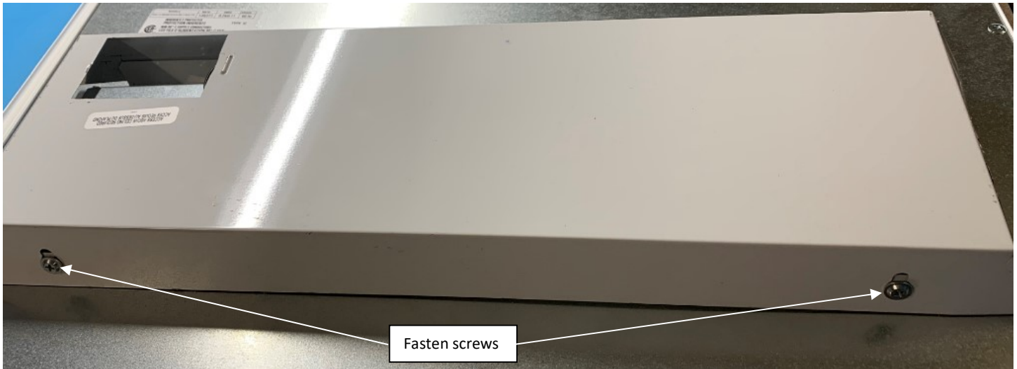
Figure 14: Fasten into place with 2 screws after sliding it in place
