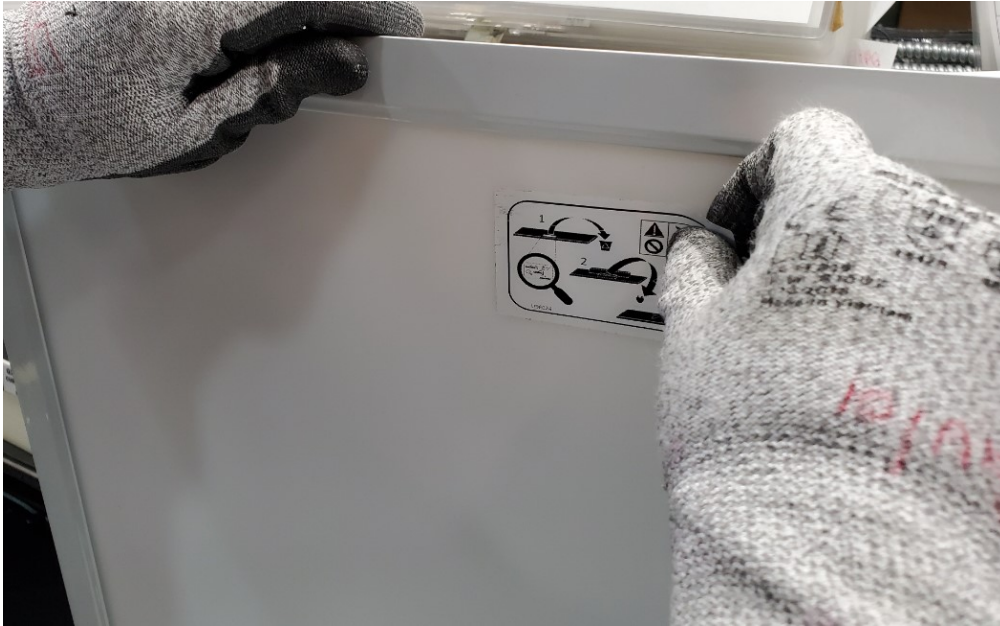
Figure 16: Remove label before RES7 installation
