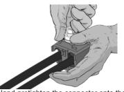
Hand-pretighten the connector onto the cables.
