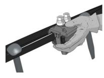
Place the 'Main' interface of the connector onto the main conductor.
