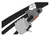
Ensure the tap cable is fully inserted into the cap, continuing until it reaches a stop.
