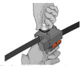
Hand-pretighten the connector onto the cables.
