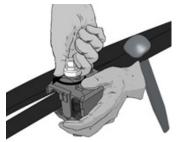
Hand-tighten the connector onto the main cable until it maintains its position.
