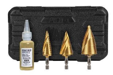
The Electrician's Step Bit Kit features three commonly used step bits, with dual spiral fluting to help pull the step bit through material for faster cutting. Titanium Nitride coating extends the life of the cutting edge. Convenient to use with an impact driver and drill, the 1/4-Inch hex shank provides a firm, positive grip. Kit comes in a rugged case that includes a convenient oil bottle for bit lubrication and longevity.
