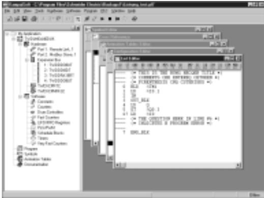
TwidoSoft is a graphical development environment for creating, configuring and managing applications for Twido programmable controllers. TwidoSoft is a 32-bit Windows-based program which runs on a PC with Windows 98 (second edition), 2000 or XP operating system. TwidoSoft software is based on a standard interface which offers the user-friendly features of the Windows environment with which users are already familiar: windows, toolbars, pull-down menus, balloon tips, context-sensitive help, etc.
