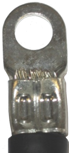
Close up of “M” Profile Crimp
