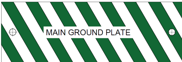
FAA1 = MAIN GROUND PLATE* Alternating Green and Clear stripes
