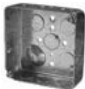
4" square standard steel box 4" x 4" x 1-1/2" (102mm x 102mm x 38mm)
