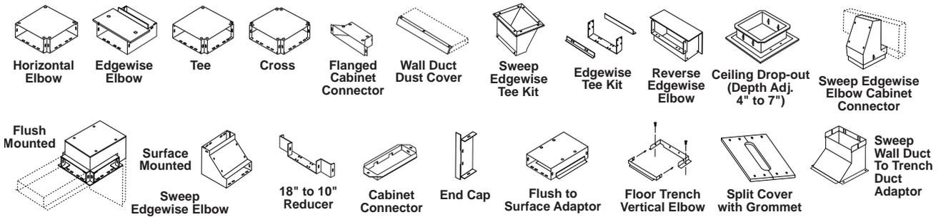
**Table 13.5: Lay-In Wall Duct Components [1] [2]**
