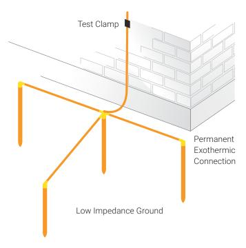
The ground electrode system should be corrosion resistant and bonded to the structural ground system. Copper and copper-bonded steel are the most common materials used for grounding conductors. Mechanical coupling can be used to join ground conductors, but suffers from corrosion effects when dissimilar metals are involved. In addition to mechanical strength, nVent ERICO Cadweld connections provide excellent, low-impedance and long-life electrical connections with excellent corrosion resistance.
