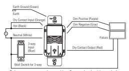
Only one sensor can be used in a 3-way circuit with a switch
