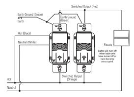
CAUTION: If a room is wired for two circuits using two separate hot leads, it is very important to connect only one circuit per relay. Both circuits must be fed from the same phase.
