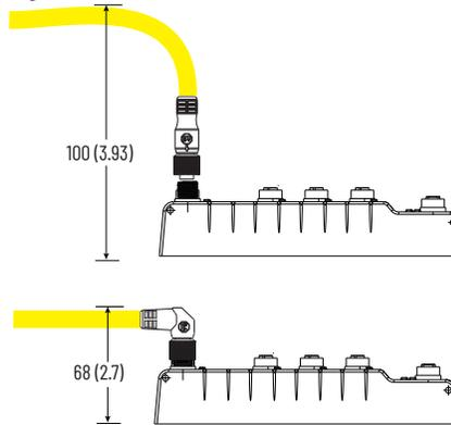
[Figure 11](#) shows an example of the 432ES-IG3 network interface module that is mounted against a side wall with all cables using right-angle quick-disconnect connectors.
