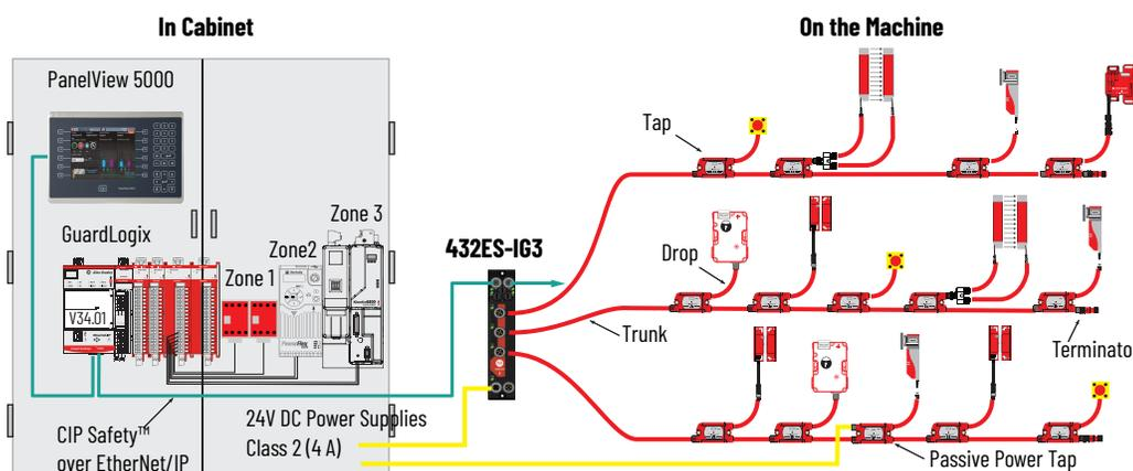
432ES-IG3 network interface module can control up to three safety zones, one zone for each GuardLink channel. With logic, the channels can combine to control only one or two zones.
