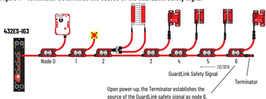
The terminator affects the closest GuardLink-enabled device. As of the date of this publication, the device can be a Smart Tap or a 440G-MZ guard locking switch. Additional GuardLink-enabled devices will be available in the future.
