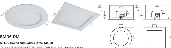
The Halo Surface Mount LED Downlight (SMD) is an ultra-low profile surface mounting luminaire with a modern look and high performance. SMD6-DM (6" with spring clips) is designed for new installation into drywall, without any additional housing or junction box needed. Suitable for residential or commercial installations. Ideal for general areas, closets, storage areas, attics and basements. Compliant with NFPA® 70, NEC® Section 410.16 (A)(3) and 410.16 (C)(5).
