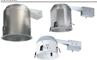
Remodel housings simplify installation when fixtures need to be added to existing ceilings. They can be installed from below in existing ceilings by cutting a precise hole, bringing power to the fixture and installing the housing. The spring clips or speed clamps lock the fixture in place. The integral thermal protector provides positive protection against overlamping. Housings are available in Insulated Ceiling (IC), Non-Insulated Ceiling (Non-IC), Air-Tite (AT) and shallow models.
