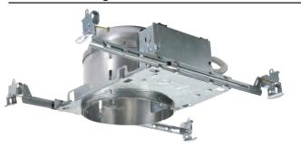
Shallow housings are designed to solve installation problems where lower joist construction is used in the ceiling. These housings accept a wide variety of trims for different lighting effects. Shallow housings are available in Insulated Ceiling (IC), Non-Insulated Ceiling (T) / (Non-IC), and Air-Tite (AT) models.
