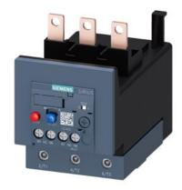
Overload relay 36...50 A Thermal For motor protection Size S3, Class 10 Contactor mounting Main circuit: Screw Auxiliary circuit: Screw Manual-Automatic-Reset
