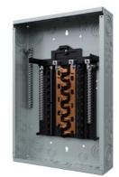
SIEMENS LOW VOLTAGE PLUG-ON NEUTRAL READY PRO SERIES ASSEMBLED LOAD CENTER. MAIN LUG WITH 20 1-INCH SPACES ALLOWING MAX 40 CIRCUITS. 1-PHASE 3-WIRE SYSTEM RATED 120/240V (125A) 100KAIC. SPECIAL FEATURES: COPPER BUS, GREY TRIM NEMA TYPE 1 ENCLOSURE FOR INDOOR USE.
