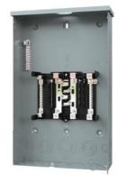
SIEMENS LOW VOLTAGE PLUG-ON NEUTRAL READY STANDARD SERIES ASSEMBLED LOAD CENTER. MAIN LUG WITH 8 1-INCH SPACES ALLOWING MAX 16 CIRCUITS. 1-PHASE 3-WIRE SYSTEM RATED 120/240V (200A) 100KAIC. SPECIAL FEATURES: ALUMINUM BUS, FEED THRU LUGS, GREY TRIM NEMA TYPE 3R ENCLOSURE FOR OUTDOOR USE.
