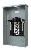
SIEMENS LOW VOLTAGE PLUG-ON NEUTRAL READY STANDARD SERIES ASSEMBLED LOAD CENTER. MAIN BREAKER WITH 16 1-INCH SPACES ALLOWING MAX 32 CIRCUITS. 1-PHASE 3-WIRE SYSTEM RATED 120/240V (100A) 22KAIC. SPECIAL FEATURES: ALUMINUM BUS, GREY TRIM NEMA TYPE 3R ENCLOSURE FOR OUTDOOR USE.
