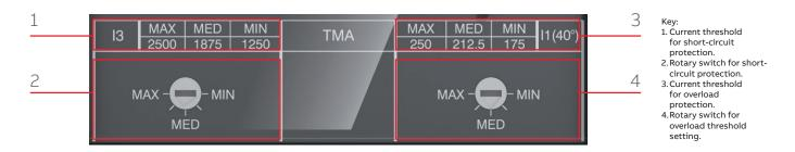
The thermal-magnetic trip unit is an easy solution for protection against overloads and short circuits. Overload protection is ensured by the ABB thermal device, based on a temperature-dependent bimetal heated by current. Protection against short-circuit is realized with a magnetic device.
