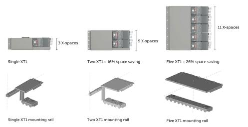
The small footprint of the XT1 allows this panel to offer multiple options to improve circuit breaker density. As you configure and order ReliaGear neXT panelboards, you'll notice that XT1 are grouped in quantities of one, two or five. As part of this feature, unique mounting brackets are required when adding XT1 breaker assemblies. See above for X-space and mounting brackets required. These additional rails are not included with SuperBox configurations and must be ordered as accessories.
