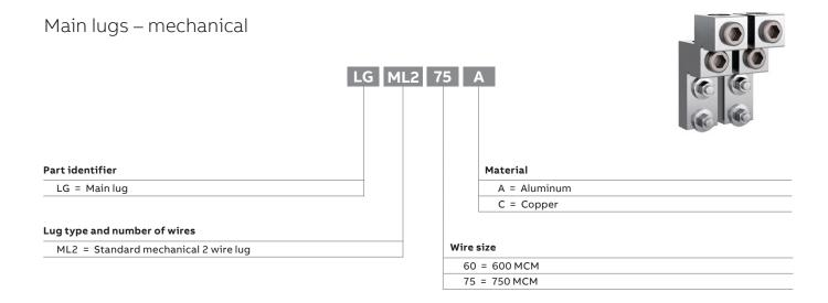
Note: \* Each catalog contains a single lug. The quantity should be multiplied by the number of phases (2X for single phase, 3X for 3 phase, and the quantity is doubled if feedthrough is needed). Also, this total quantity should be multiplied by 2 if there are 2 lugs needed per phase.
