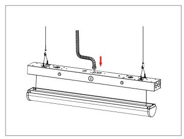
6. Secure the LED Cover to the Housing by Pressing upward and lock it with springs tightly located into the fixture.
