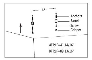
2. Then, tighten gripper back to the barrel and adjust to desired length of cable. Clip-on to the keyholes of the fixture.
