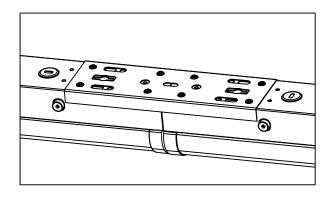
6.Take the black/white/green wire harness and connect to the existing wire connectors on the input wires of the driver respectively. When using the dimming function, take the purple and gray wire harness and make connection to driver with connectors included in the parts pack. Please make wiring connection using the wiring diagram.
