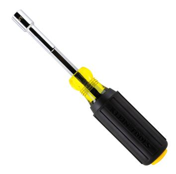
Klein's Color-Coded Hollow-Shaft Heavy-Duty Nut Driver features a fully pass through driver for driving nuts on threaded rod and prevents bottoming out. Cold forged steel wrench assist provides greater torque, especially helpful for breaking stubborn nuts and bolts free. The handle is ASME color-coded and dome-stamped to easily identify the common 5/16-Inch hex size needed for the job.
