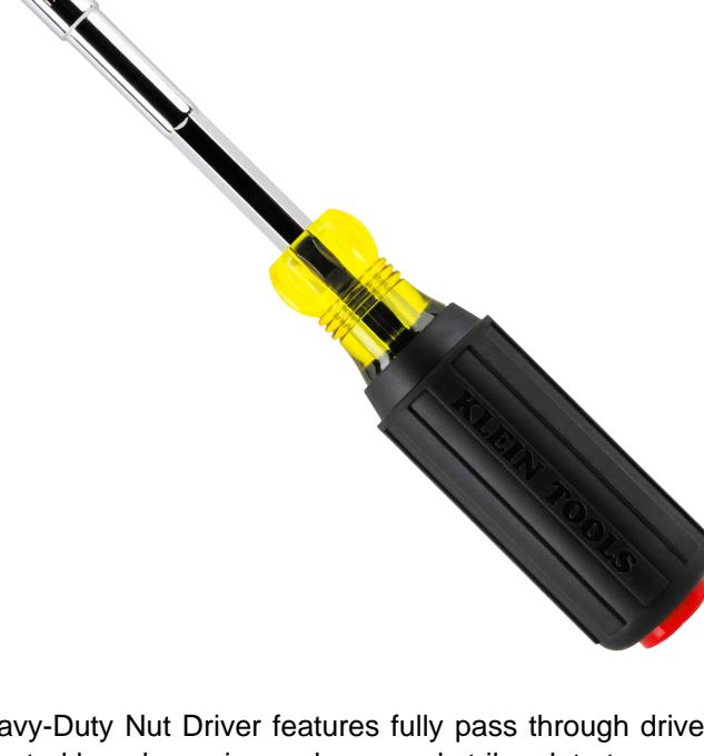
Klein's Magnetic Color-Coded Hollow-Shaft Heavy-Duty Nut Driver features fully pass through drivers for driving nuts on threaded rod and prevents bottoming out. Rare-Earth metal magnet is protected by a brass inner sleeve and strike plate to prevent the magnet from falling out or being damaged by sharp edge threaded rod. Cold forged steel wrench assist provides greater torque. Color-coded handle and dome-stamped to easily identify the common 1/4-Inch hex size needed for the job.
