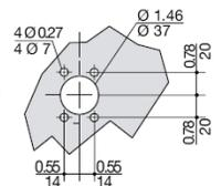
**LK4TU3N / LK4UU3N / LK4WU3N, 800–1200 A Nonfusible Disconnect Switches—Dimensions**
