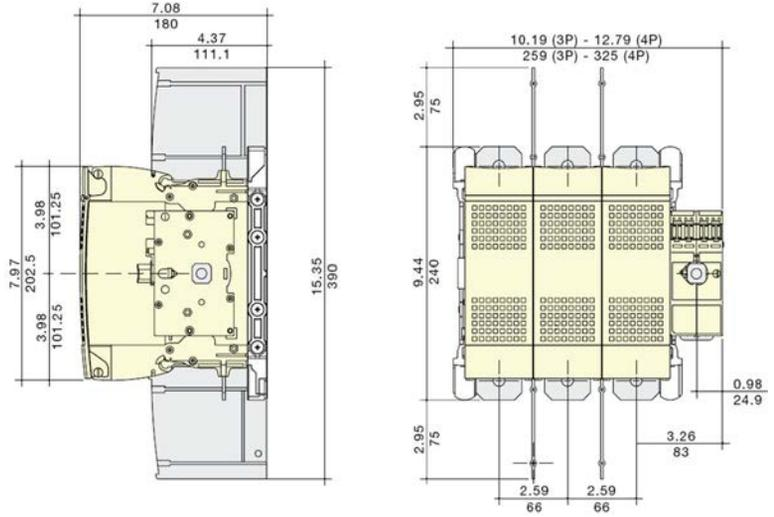
GS2SU3 600 A (Class J Fuses) and GS2TU3 800 A (Class L Fuses) Fusible Disconnect Switches
