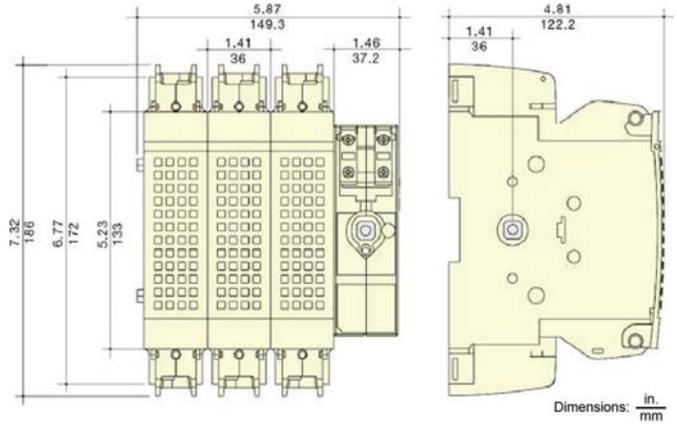
**GS2MU3N, 200 A Fusible Disconnect Switches, Class J Fuses**
