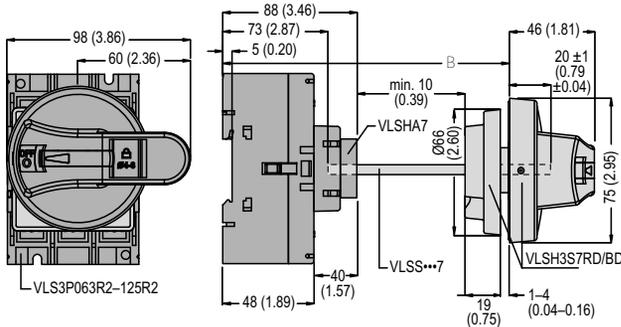
VLSS...7 used with VLS8M2 and VLSH3S7RD/BD handle
