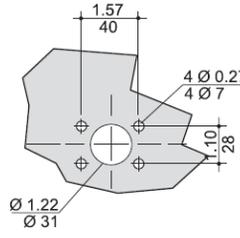
Door drilling with fixing nut
