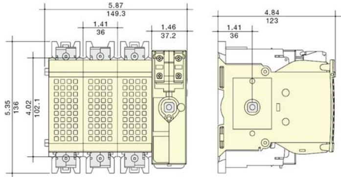
**GS2JU3N, 100 A Fusible Disconnect Switches, Class J Fuses**
