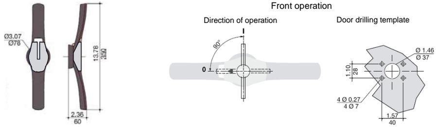
**GS1DDU3, 30 A Fusible Disconnect Switches, Class CC Fuses and GS1DU3, 30 A Fusible Disconnect Switches, Class J Fuses—Dimensions**
