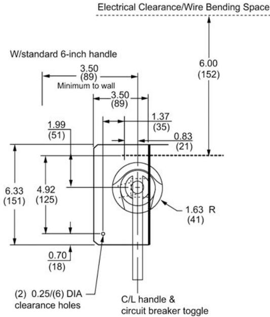
Panel Drilling for PowerPac™ D and L Circuit Breaker Operating Mechanisms: 9421LD1, 9421LD4, and 9421LD7
