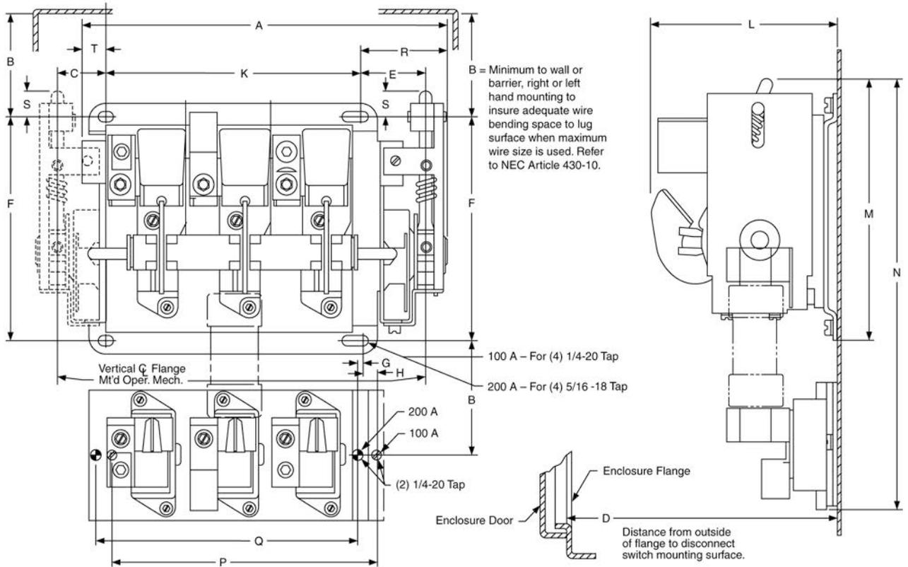
[20] The dimensions shown may be extended 7 in. by using 9422R2 (two required per switch).
