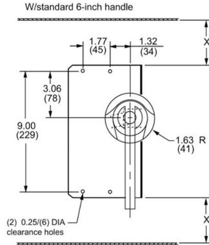
X: Minimum to wall or barrier to insure adequate wire bending space to lug surface when the maximum wire size is used. Refer to NEC 430-10.
