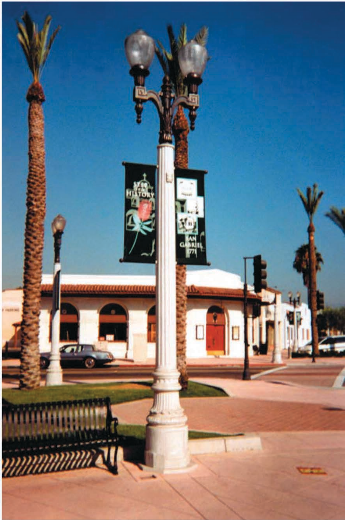
San Gabriel SG21 with SCTW Decorative Twin Arm and Modified Acorn Luminaires
