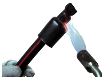
2. Beginning at closed end apply heat, blue thermochromatic lines will begin to disappear at 150° C. Gradually, move heat source to open end and around cap. Once lines are no longer visible and adhesive flows out of open end, discontinue heating.
