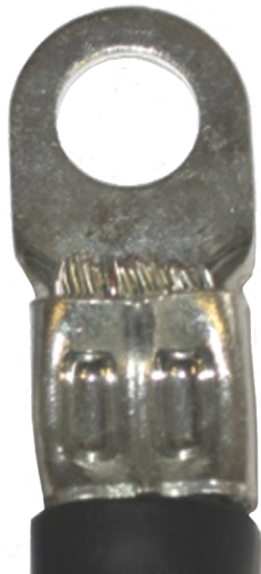
Close up of “M” Profile Crimp
