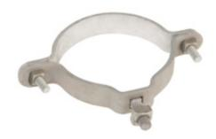
Secondary Rack Pole Band for attaching secondary racks to tubular metal poles. Band is euipped with  $5/8" \times 2"$  carriage bolt for attaching the one secondary rack. Hot dip galvanized.
