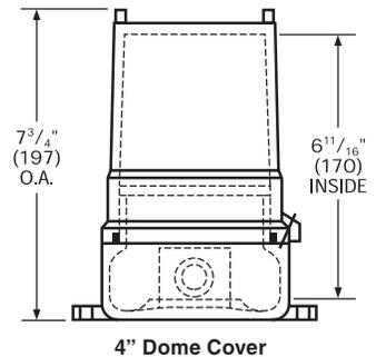
For HK1GLD (1" Dome Lens Cover), add 1" to lens cover verticle height dimensions
