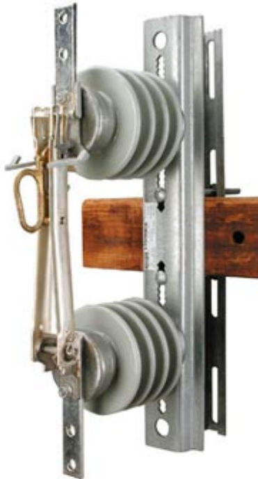
14.4kV, 110kV, 600 A, Single-Phase Hookstick Disconnect Switch
