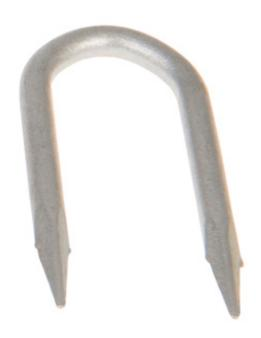
Diamond Point Staple, hot dip galvanized, 1" long x 5/16" inside width x .12" diameter wire. Used to secure ground wire and ground wire molding to wood poles.
