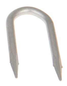
Diamond Point Staple, hot dip galvanized, 2" long x 1-1/16" inside width x .188" diameter wire. Used to secure ground wire and ground wire molding to wood poles.
