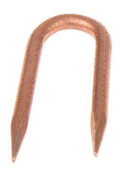
Diamond Point Staple, copper coated, 2" long x 1-1/16" inside width x .188" diameter wire. Used to secure ground wire and ground wire molding to wood poles.
