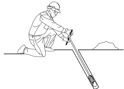
3. turn rod to expand.
