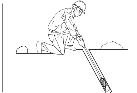
2. push anchor into hole
