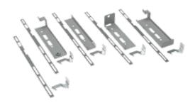
An operator adapter is required to install a disconnect in Bulletin A21S4, A28S4 and WS2D Hoffman enclosures that have a preferred cutout. Operator adapters include components needed to interlock the master door with the disconnect operating mechanism. Panel drilling and installation instructions are furnished with each operator adapter.
