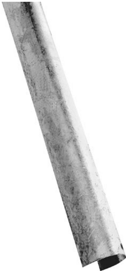
U-Cable Guard 1 1/8" inside diameter x 5' long. Protect telephone and powerlines where circuits lead from underground to overhead. Guards are 14-gauge hot dip galvanized steel, formed into "U" shape. RUS Listed
