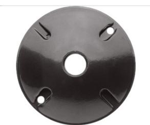
Die cast round covers with one or three 1/2" holes. Fit 4" round boxes. Supplied with thick foam rubber gasket and two #10-24 stainless steel screws. 3 hole cover comes with one die cast 1/2" close-up plug.
