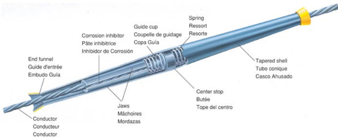
Inside an Automatic Splice.
