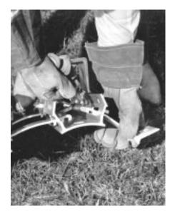
Adjust hook plates as necessary: remove locking spring, move hook plate to proper notch, and reinstall locking spring. Check mounting brackets and hook plates for proper assembly before proceeding with installation.
