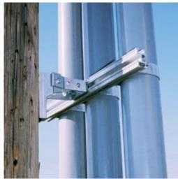
Aluminum Conduit Standoff Bracket and T-Slot, mounts 1" to 6" conduit with unlimited adjustability. No field drilling required. Mounts to pole on 3 5/8" centers using 5/8" through bolts and 1/2" lag, not supplied. Conduit straps are ordered seperately for specific sizes. Additional T-Slot shapes can be ordered seperately.
