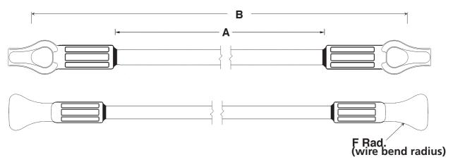
5/8" dia. Fiberglass rod. Castings are hot-dip galvanized ductile iron.
