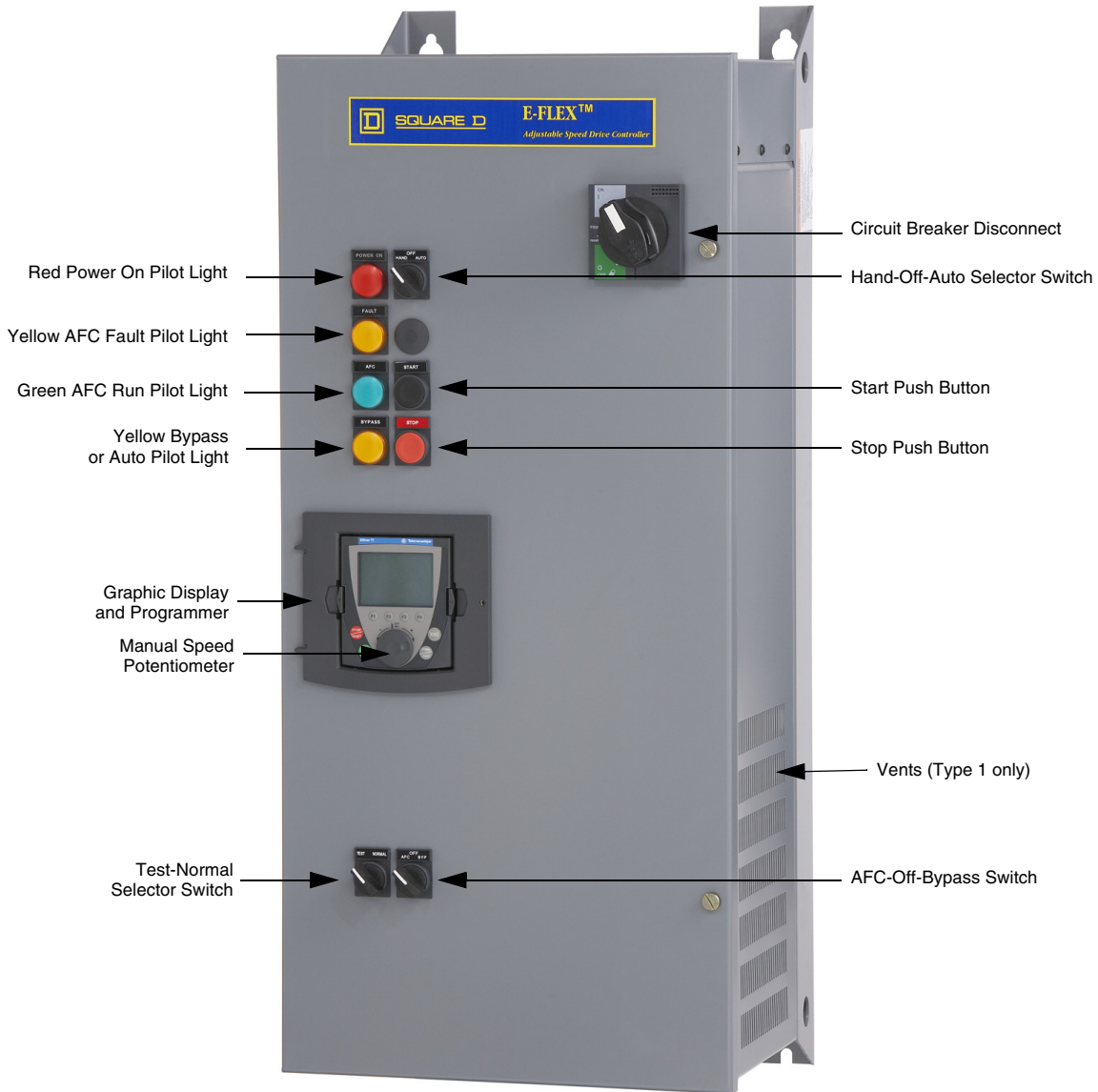
Figure 2: Typical Type 1/12K Front Component Locations for Controller: 1–100 hp @ 460 V and 1–50 hp @ 208/230 V (Class 8839 Type EFDG4VY, Mods: B07, B08, A09, C09, E09, and P09 shown)
