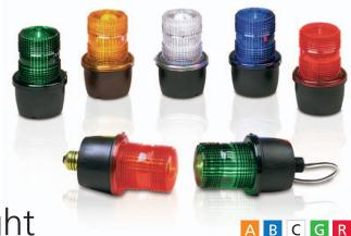
Model LP3 is offered in three mounting configurations. The LP3S features a three-hole surface mount — ideal for control panels and other flat or flush surfaces. The LP3E features a standard A-19 medium Edison screw-in base. The LP3M features a 1/2 " NPT male pipe mount and 18 " wire leads.
