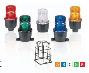
Model LP3 is offered in three mounting configurations. LP3P features an integrated 1/2-inch NPT pipe mount. LP3S features a three-hole surface mount — ideal for control panels and other flat or flush surfaces. The "T-mount" LP3T has a popular 2-hole design for wall or flush mounting.
