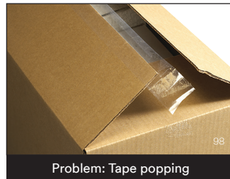
Problem: Tape popping
