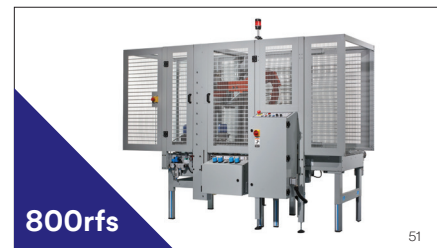
800rfs 3M-Matic™ Case Sealer 800rf Type 40800 is a fully automatic random size case sealer that automatically adjusts for various case sizes and folds the top minor and major flaps up to 10 cases per minute. Using tape widths from 36mm to 48mm tape widths.
