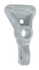
Pole Eye Plate, cast ductile iron, has eye for maximum 3/4" diameter pin. Cast integral lag spur prevents rotation.
