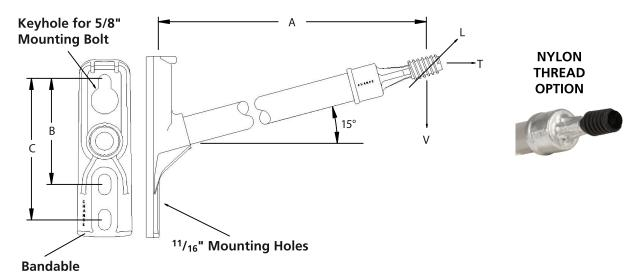
**B** Dimension is 6" for 1SBM series and 8" for 1SBH series **C** Dimension is 8" for 1SBM series and 10" for 1SBH series
