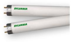
General25W, 36" MOL, T8 OCTRON XP Extended Performance fluorescent lamp,Description:3500K color temperature, rare earth phosphor, 85 CRI, suitable for IS or RS<br/>operation, ECOLOGIC®3
