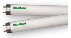
General32W, 48" MOL, T8 OCTRON fluorescent lamp, 3000K color temperature, rareDescription:earth phosphor, 85 CRI, suitable for IS or RS operation, ECOLOGIC
