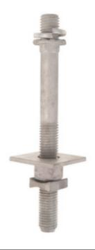
Serrated collar and lockwasher secure unit to line post insulator and prevent accidental disassembly. Cut threads above serrated collar, rolled threads below collar.
